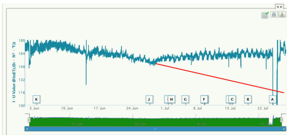
Figure 3. Graph of the U-value of the MEA cooler over time. After the trend was realised, chemical adjustments were made that helped recover efficiency.
